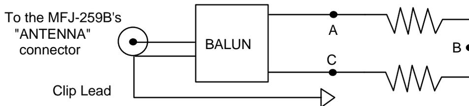
A properly designed current balun is the type most effective for maintaining current balance. It has the highest power capability and lowest loss for given materials. It should show a low SWR over the entire operating range of the balun with the clip lead in any of the three positions.
